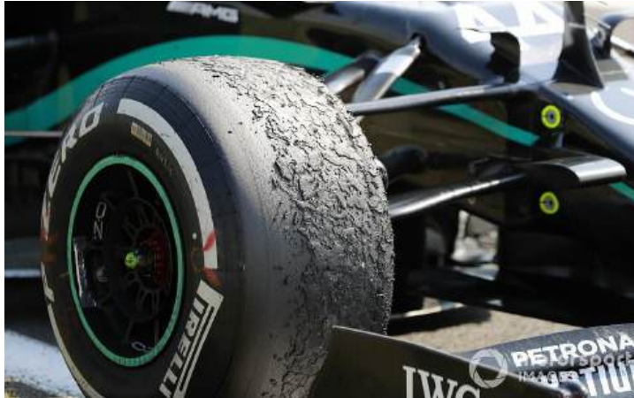
Figure 2: Worn wheel at the end of the race with rubber debris from the asphalt, that can't be reused or recycled
