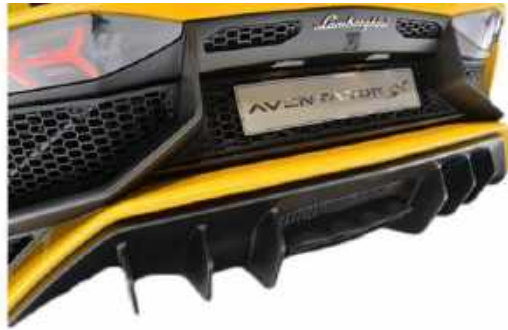
Figure 2. Image of a diffuser present on a Lamborghini Aventador SV, reprinted from Ref. [4].
