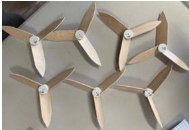
Figure 3. The seven different 3-blade designs of different installation angles (30°, 35°, 45°, 50°, 55°, 57.5°, 60°, C-Type)
