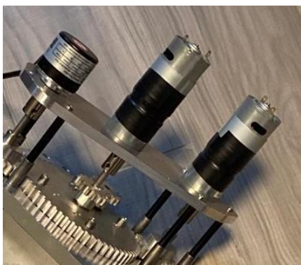
100RPM DC motors used in swerve module
