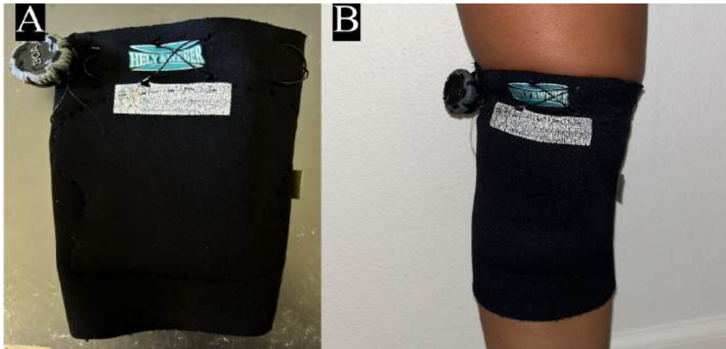
Figures 3: (A) Rapid Prototype Knee Sleeve With Inserted Knee Padding and Weaved BOA® Adjustment System. (B) Prototype on A Player's Knee
