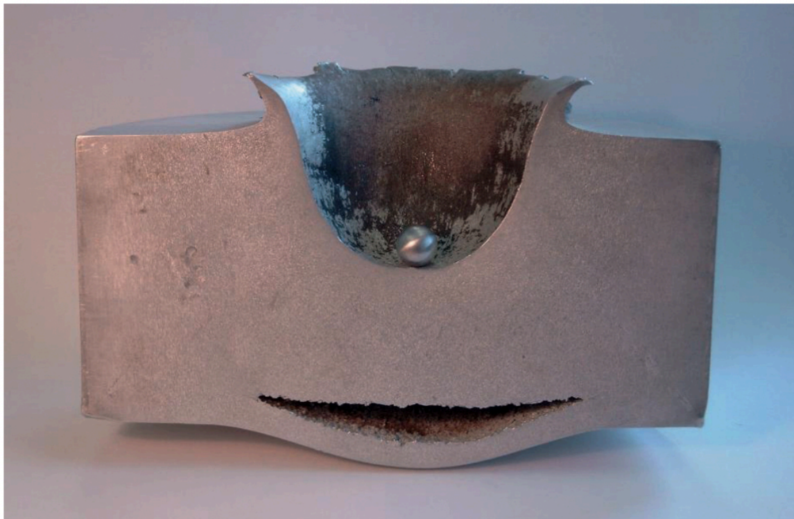
Figure 1: Results of the experiment conducted by the ESA on the power of Space Debris
