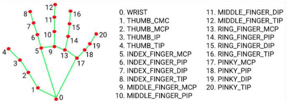
Figure 2: Specific key points “name” and the index to find them when retrieving all data points[6].
