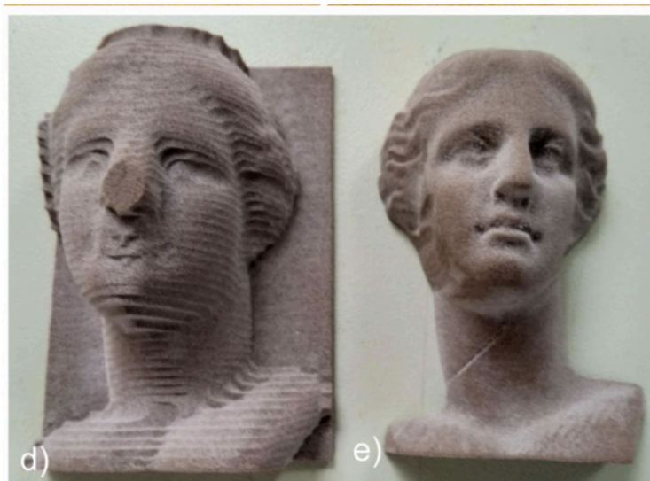
Fig 2: Reproduction using subtractive technology on a Sica block [Zivanovic et al. 249].
