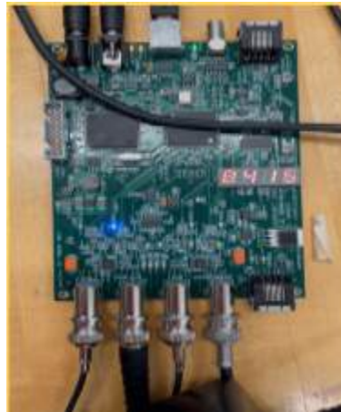
Fig 4. Circuit used to detect muon counts
