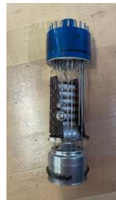
Fig 3. Photomultiplier used in the experiment
