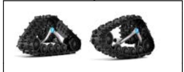
Fig. 6. Left: Camso X4S back tracks. Right: Camso X4S front tracks [4]
