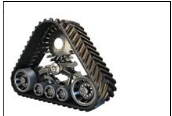
Fig. 7. PowerFlex Trax back tracks. [5]
