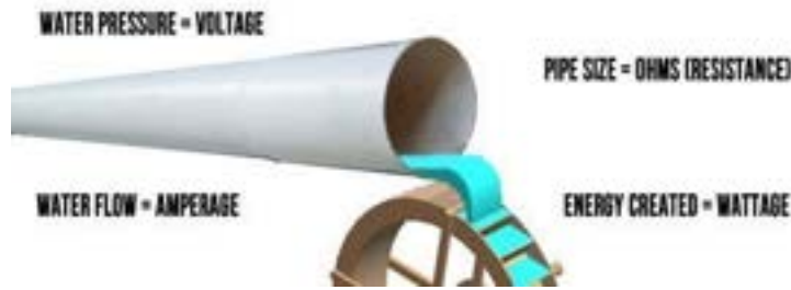
Figure 1: Water Pipe Analogy for Understanding Electricity (“Understand Power”)
