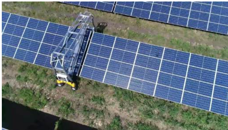
Fig 2: Image of SolarCleanO B1 at work in a Solar Array. From https://www.youtube.com/watch?v=omZRKmPLQcQ
