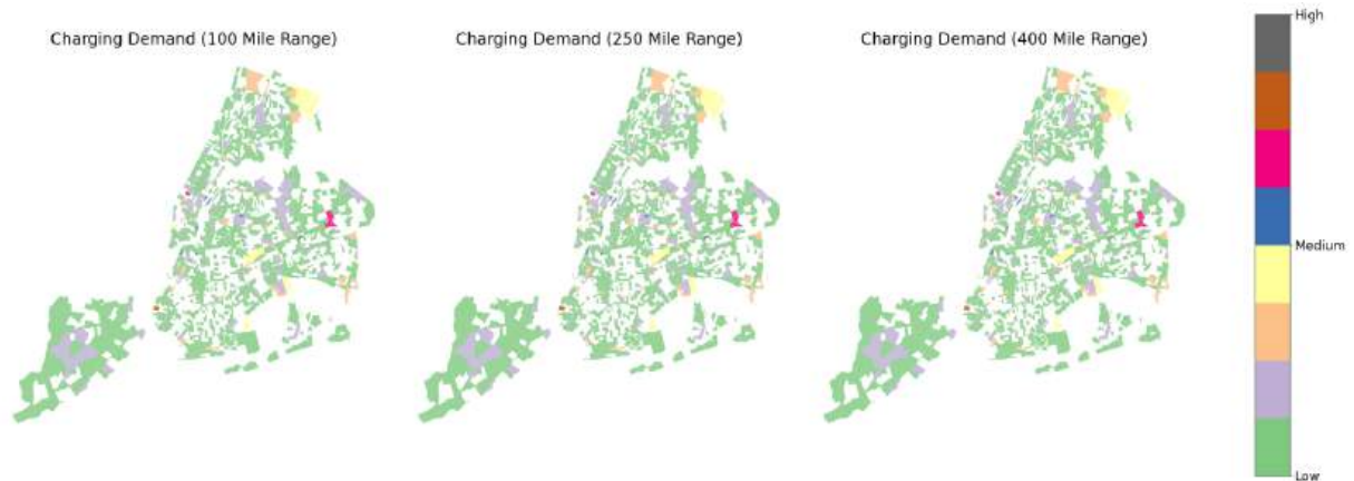
Fig. 5. Spatial Distribution of EV Charging Demand in NYC for 100, 250, and 400 Mile Range Vehicles. I used the NYC OpenData Traffic Volume Counts dataset to create the maps of EV charging demand for 100, 250, and 400-mile range vehicles, as shown in Fig. 5. These maps illustrate the spatial distribution of charging demand across New York City, highlighting how different vehicle ranges influence the areas where charging infrastructure will be most critical, with longer-range vehicles requiring fewer but more strategic station placements in high-demand regions.
